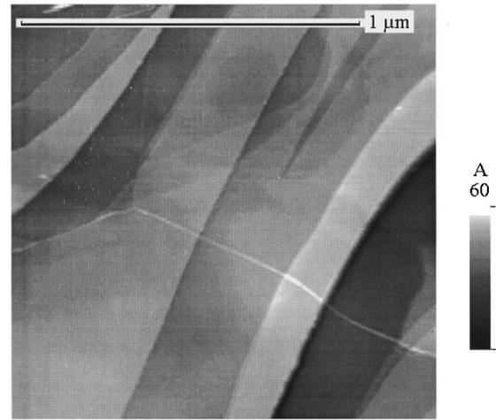
FIG. 2. Constant current plane view image of a single nanotube from an *A* type sample, crossing a plateau with two unequal steps on both sides. The apparent tube width is in the 160-Å range, while the apparent height of the tube is in the 8–9 Å range. See dimensions in Fig. 4 and Table I.
