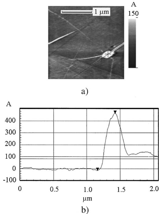
FIG. 1. Constant-current STM image of carbon nanotubes of a 10-nm diameter in a *B* type sample. (a) Plane view image; note the light object (marked with a cross in the center) from which emerge three nanotubes. (b) Line cut along the black line shown in part a; the protruding “hill” of 460 Å corresponds to the tip shape; note the plateau in the line cut on the right-hand side of the “hill” which corresponds to the height of the nanotube.
